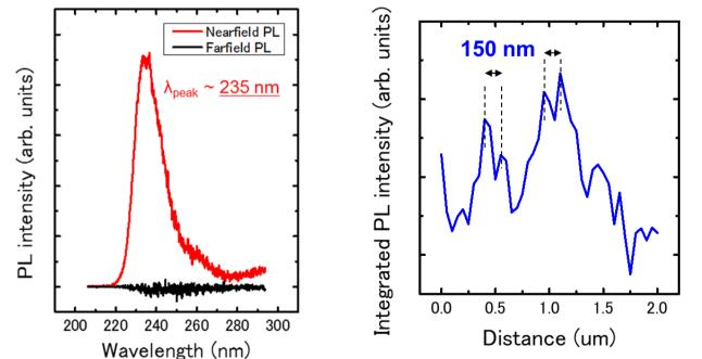
With **<u>210 nm</u>** excitation wavelength, below 240 nm emissions from AlGaN QWs can be measured.
