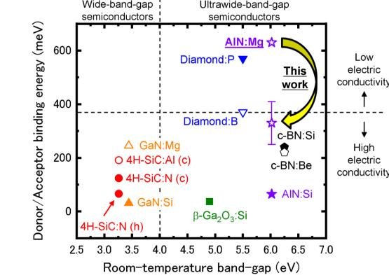
Our high-resolution DUV photoluminescence spectroscopy deduced an **unexpectedly small** Mg acceptor binding energy of AIN.
